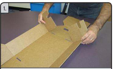
Starting with the "Base" (shown in the components list above), pre-break all score lines. After pre-breaking scores, fold in "minor flaps" on one end to come together.
