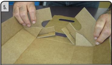
Now pre-break all score lines on the "Lid" (shown in the components list). After pre-breaking scores, begin to fold "minor flaps" in while making sure the "ears" and "slot flaps" are both folded inside.
